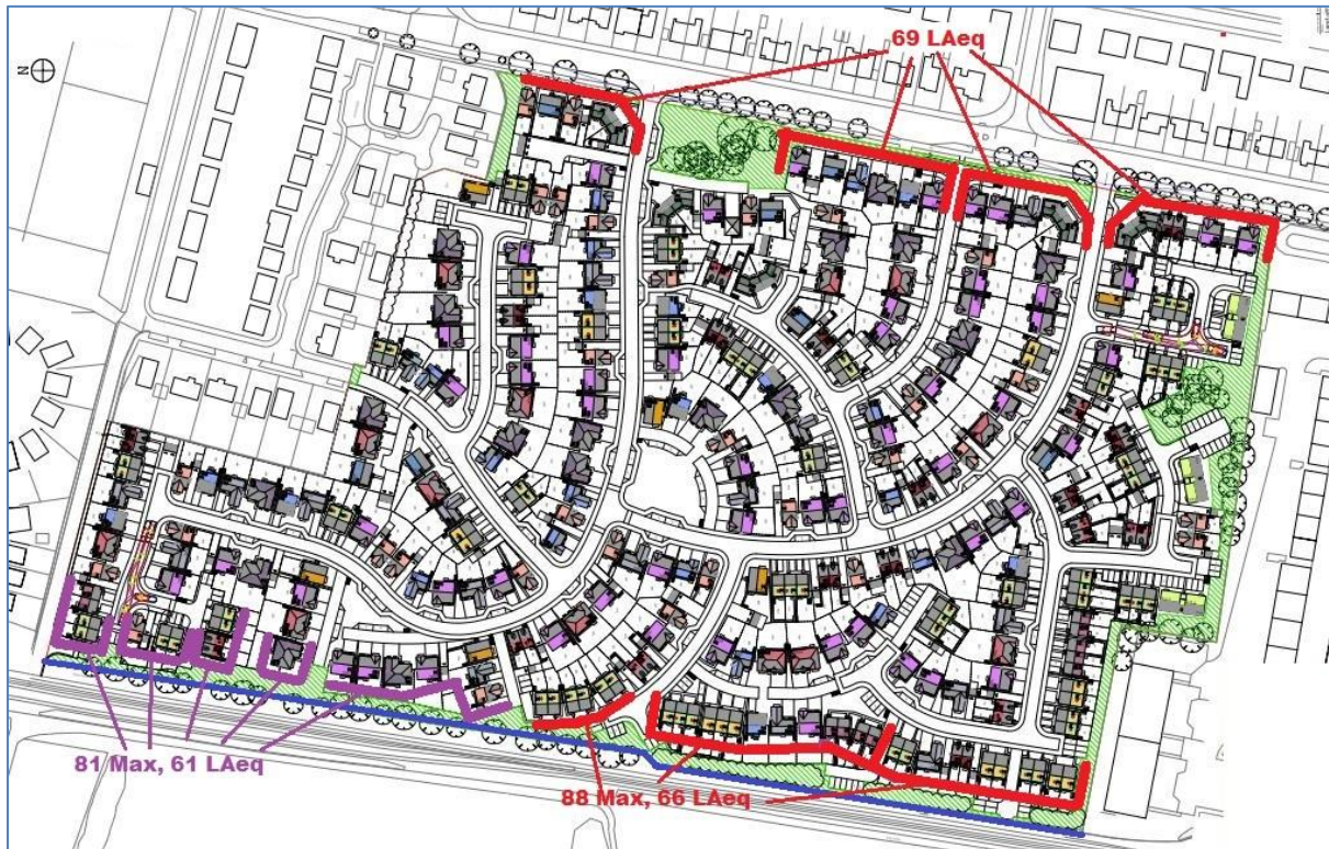
Figure 3: Proposed Development – Expected Worst Case 1 st Floor Façade Noise Levels (Road and Metro)
