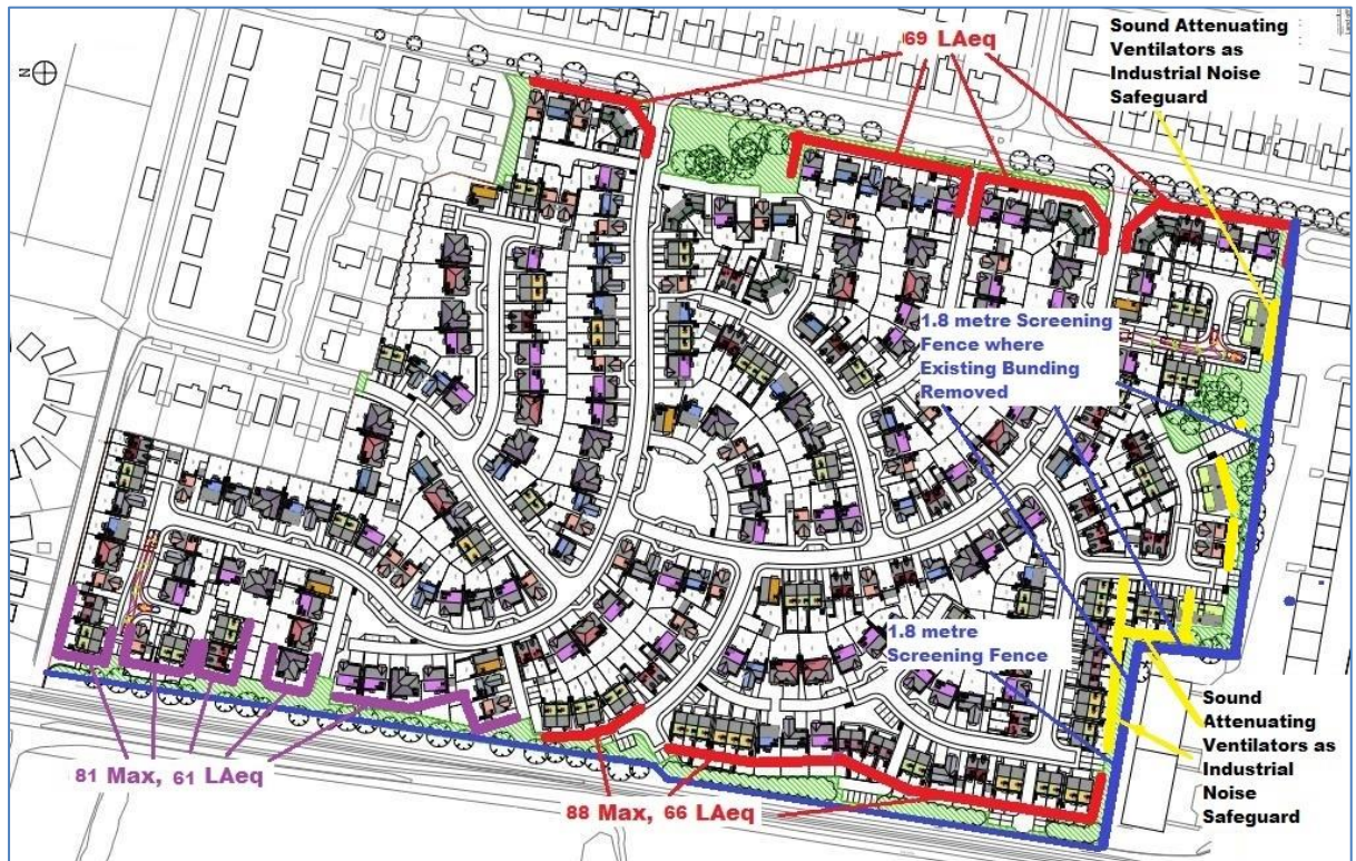
Figure 9: Recommended Addition Amelioration Measures re Potential Industrial Noise
